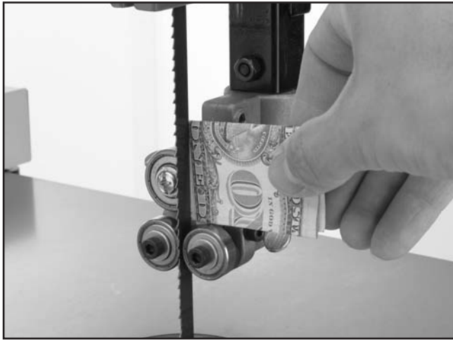
Figure 21. Dollar bill folded twice to make a quick .016" gauge.
